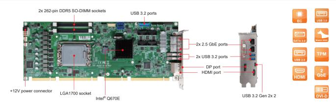
ROBO-8116G2AR is based on Intel® 600 series chipset and workstation processors. Built with flexible PCI express expansions, ROBO-8116G2AR is suitable for Medical, Industrial automation, and Digital Signage application.
